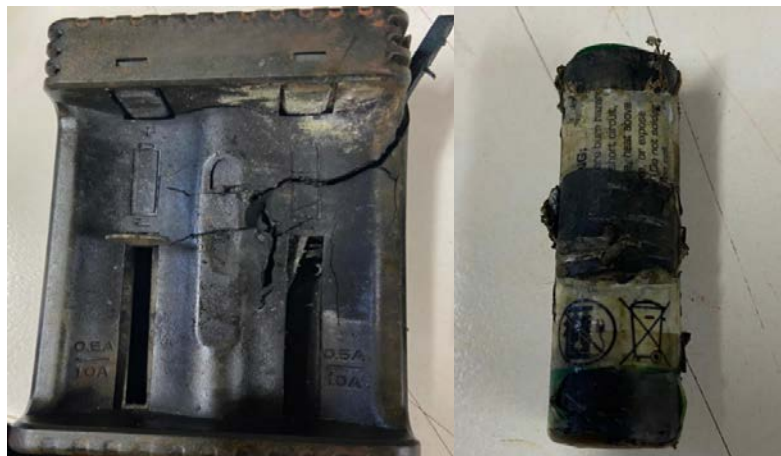
Figure 3: Thermal runaway incident from non-rechargeable Li-ion battery inserted into a charger
