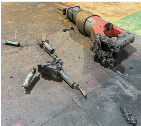
Figure 1: Handheld power tool Li-ion battery fire
