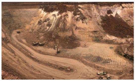
Multi-bench pit wall failure. Note the vehicles in the vicinity of the wall failure.
